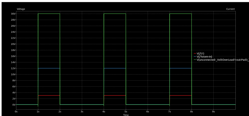
Fig. 5: Spice Simulation in KiCad for 1xV Totem-Pole Switching
