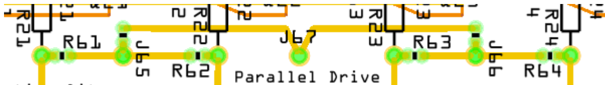
Fig. 7: The option for driving the MOSFETs in parallel, by shorting R31-R64, and J65-J66.
